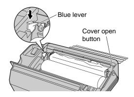
2 Cut off the wrinkled portion, and replace the recording paper roll in the proper direction.
